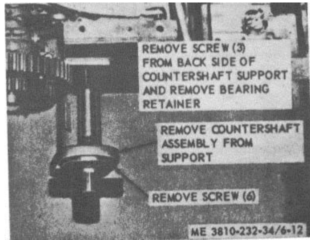
Figure 6-12. Crane countershaft assembly, removal and installation.
